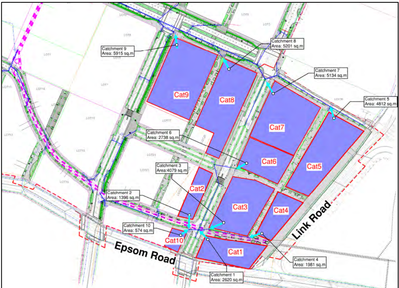
Figure 7 – Proposed Sub-Catchment Plan and Points of Discharge to the Council Stormwater System
