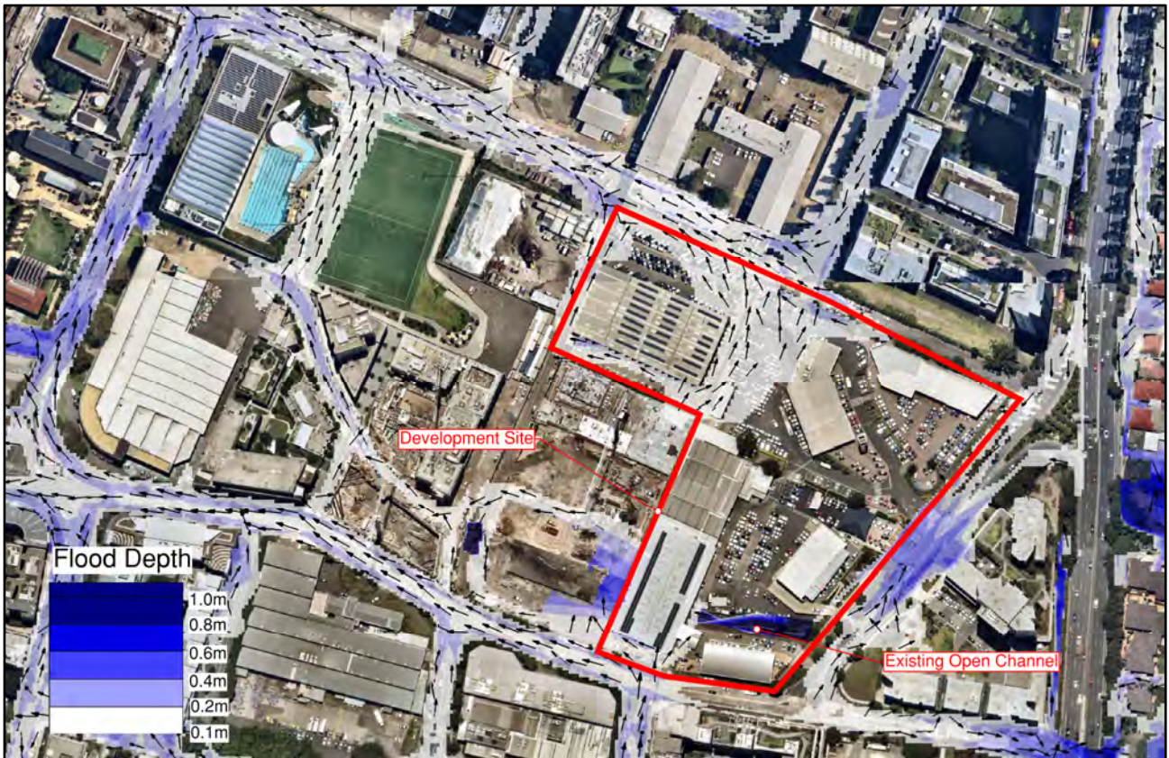
Figure 13. Existing Council 1% AEP Flood Depths Around The Development Site
